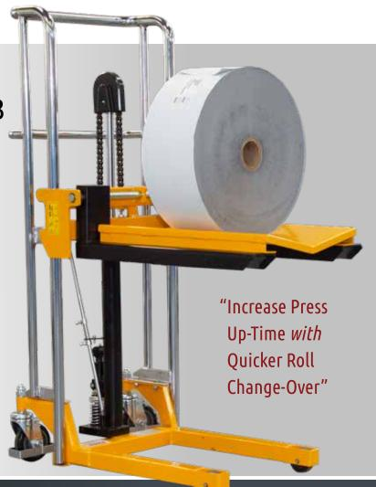
Roll tray extends 6" in front of the bottom casters for quick and easy access to roll core chucks.
