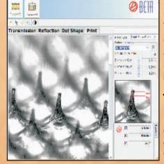
3D Imaging is the Only Way to Calibrate and Control HD Screening Techniques. Photopolymer and elastomer plates are easily imaged, analyzed, and compared to the shop standard. "Dot Structure Index" simplifies the production worker's job while detailed measurement data is available to the QC manager.
