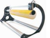
Dual transmission illuminators produce sharp, high-contrast images for accurate halftone dot analysis for the Betaflex Pro Measuring Head in both 2D & 3D modes.
