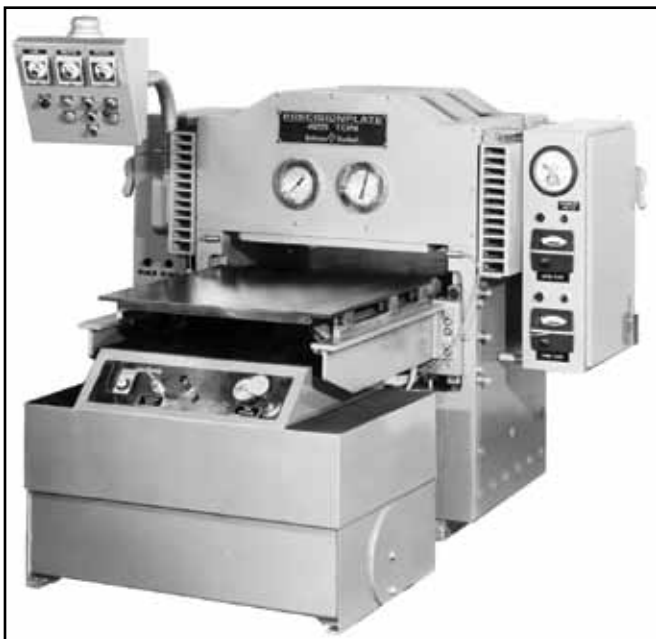
An early hydraulic molding press sold by A&V in the 1960s.
